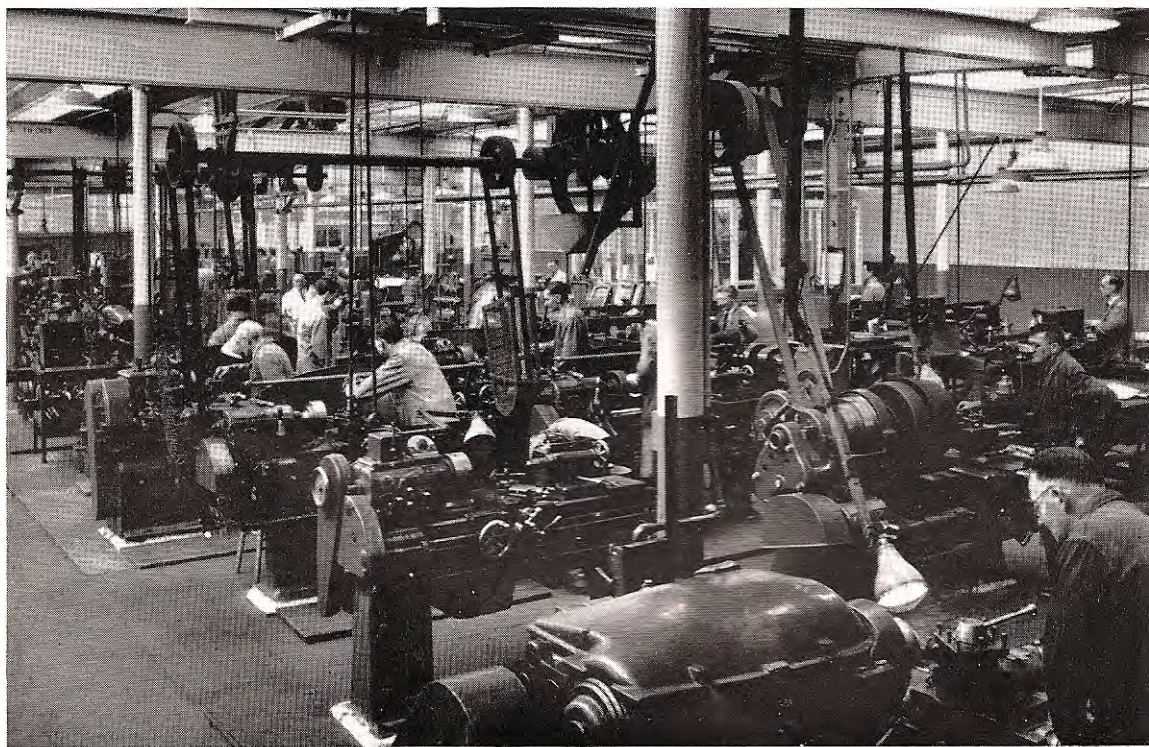
Machine Shop (Above). Part of the Machine Shop with a line of Capstans in the foreground.
