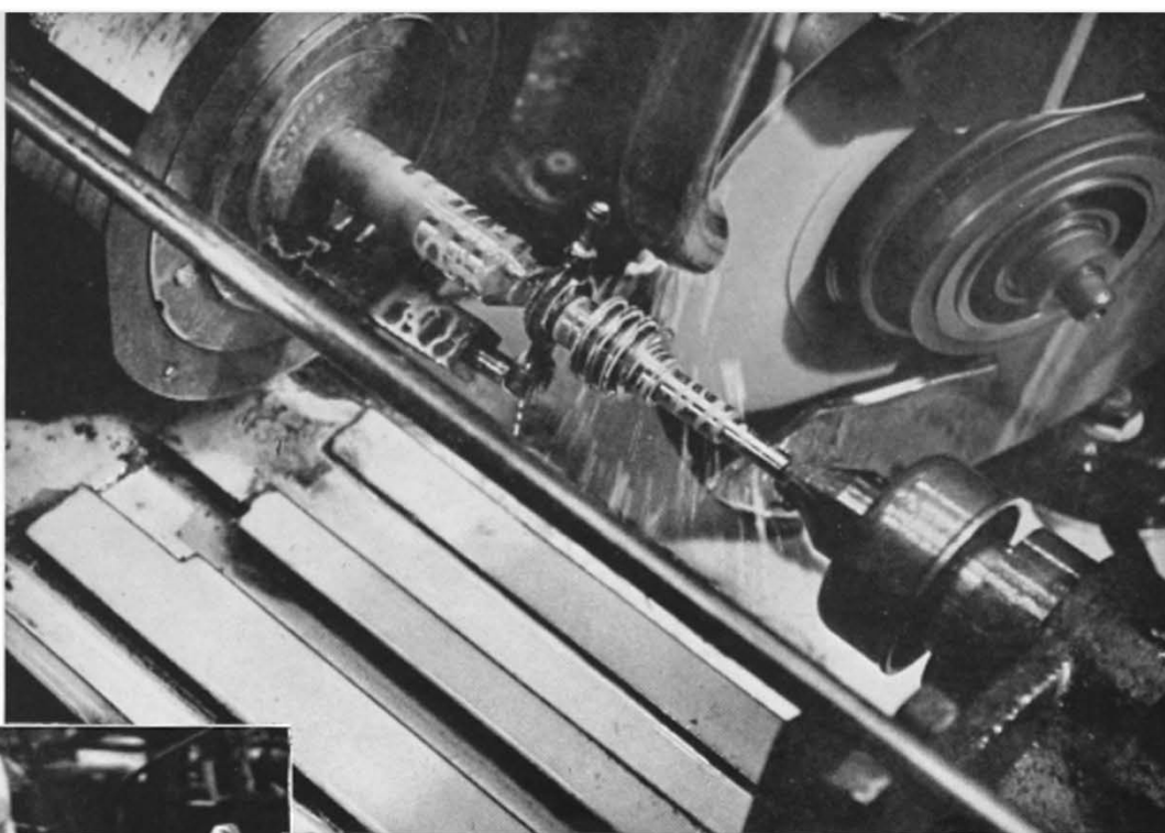
Another highly specialised job. A close-up view of worm-thread grinding.
