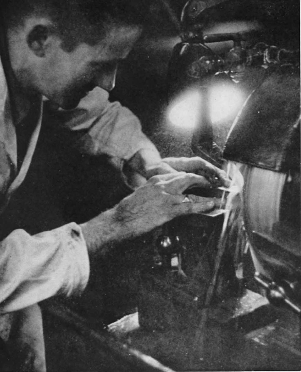
Tungsten-carbide tipped tools. Such tools are extensively used and are carefully ground and lapped on special machines to predetermined shapes.
