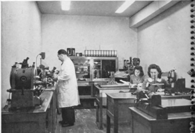
The Swift Standards Room. Kept at a temperature of 68 deg. and constant
