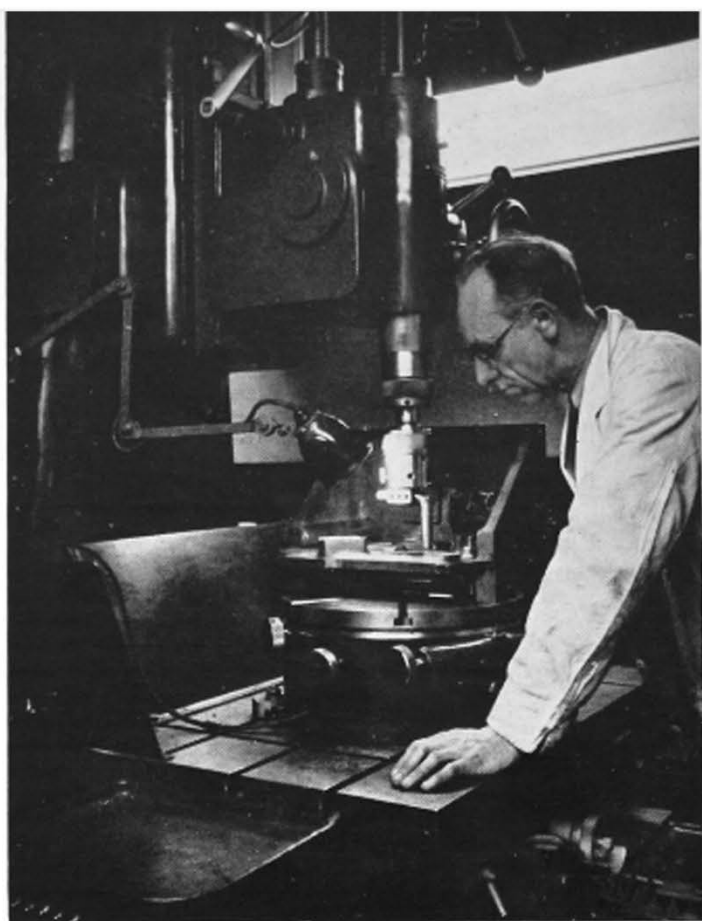
A case of extreme precision. Jig-boring in an air-conditioned, temperature-controlled room away from the noise and bustle of machine shops.
