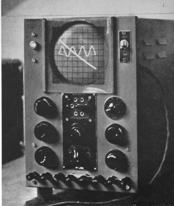
The Oscillograph. It records oscillations of time, pressure or sound.
