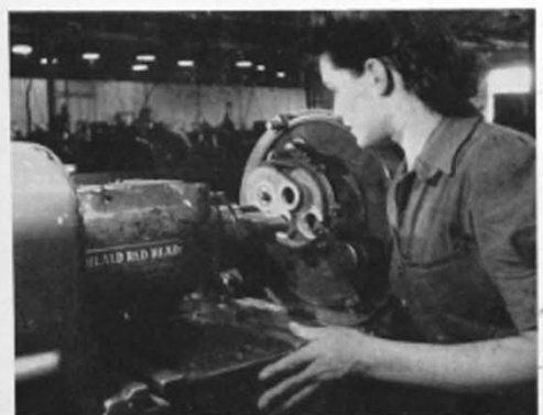
Fine Boring. For high finish and accuracy.
