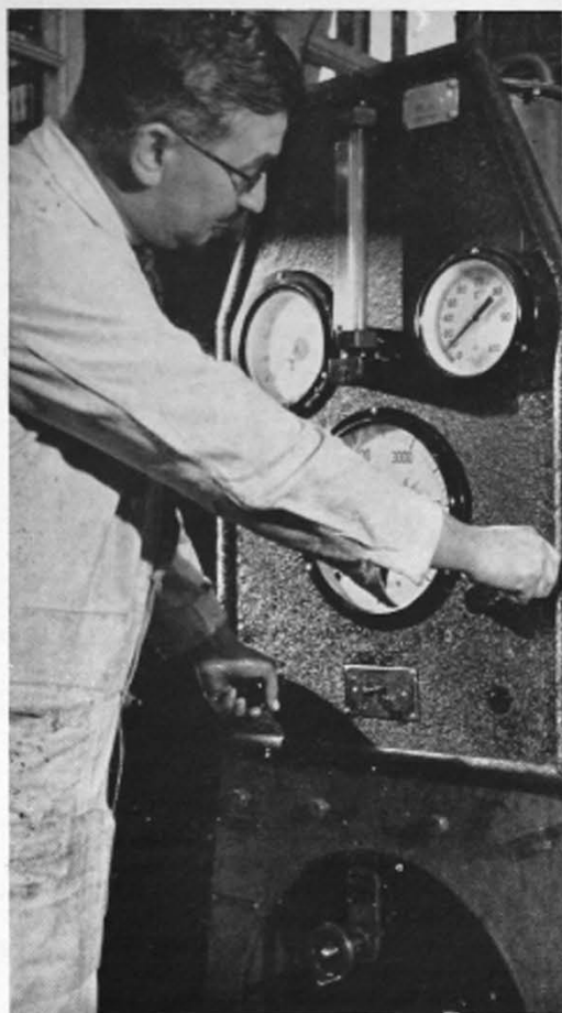
Taking the readings. Testing an hydraulic pump running at pressure.
