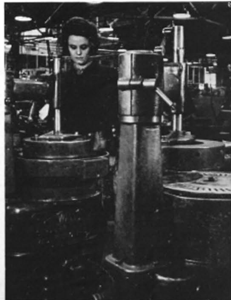
Lapping Surfaces. A high-class finish for long life.
