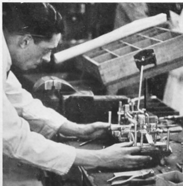
The birth of a Weighing Machine. Mechanism being assembled.
