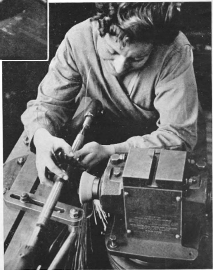
Sharpening Milling Cutters. Must be made, and kept, sharp and accurate.
