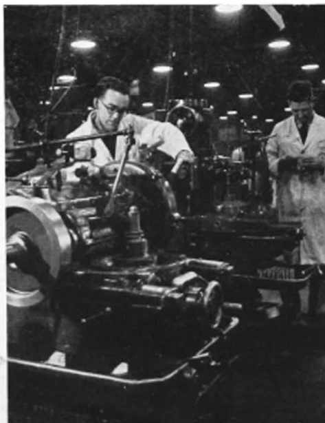
Worm-wheel generation. A high-speed machine.
