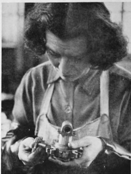
A Sub-assembly. Part of an hydraulic pump.
